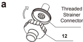
Screw the hose adaptor B (12) to the threaded strainer connector, from inside of the pool.
