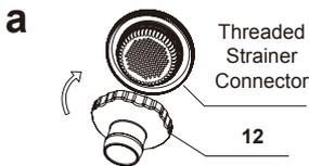
Screw the hose adaptor B (12) to the threaded strainer connector, from inside of the pool.
