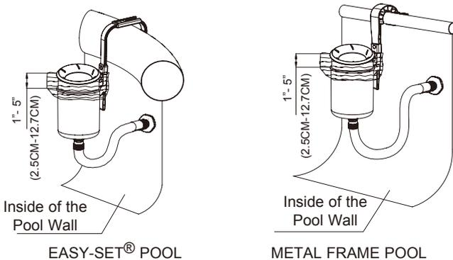
**IMPORTANT:** The skimmer must stay vertical at all times, so that the top of the floating cover can parallel to the water surface for skimming.
